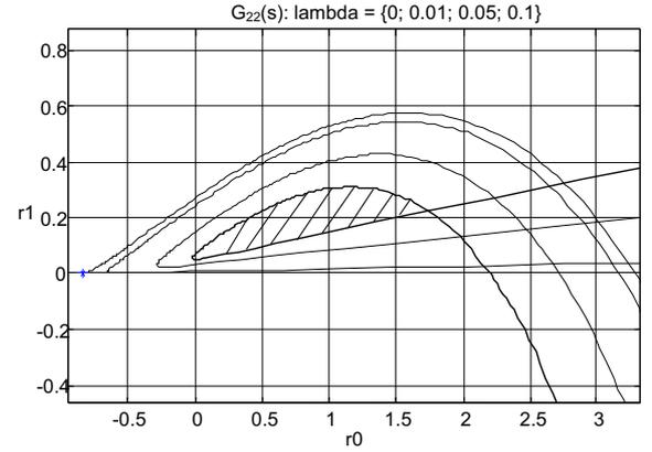
Fig. 4. Neymark D-plots for the 2nd subsystem
