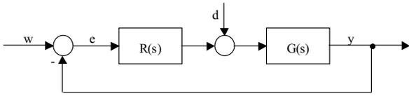
Fig. 1. Standard feedback configuration
