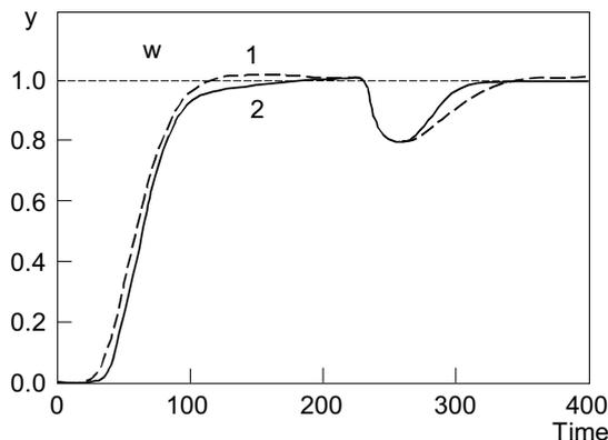
Fig. 5. Step setpoint and load disturbance responses:  $\tau_d = 24$ ,  $\varphi = 400$ . (1)-the numerator, (2)-the Padé approximation.
