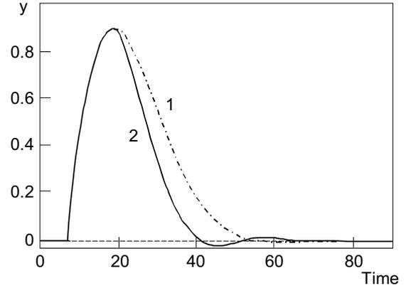
**Fig. 3.** Load disturbance responses:  $\tau_d = 8$ ,  $\varphi = 1$ . (1)-the numerator, (2)-the Padé approximation.
