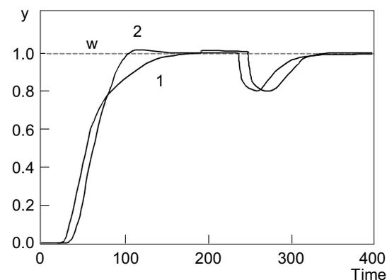
Fig. 7. Step setpoint and load disturbance responses using the Padé approximation:  $\varphi = 400$ . (1) -  $\tau_d = 19.2$ , (2) -  $\tau_d = 28.8$ .
