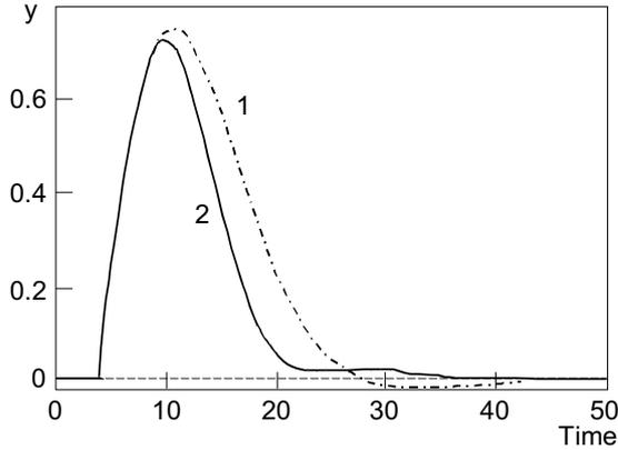
**Fig. 2.** Load disturbance responses:  $\tau_d = 4$ ,  $\varphi = 1$ . (1)-the numerator, (2)-the Padé approximation.
