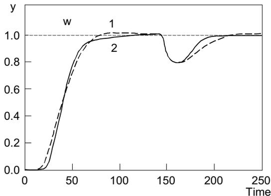
Fig. 4. Step setpoint and load disturbance responses:  $\tau_d = 16$ ,  $\varphi = 100$ . (1)-the numerator, (2)-the Padé approximation.
