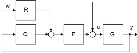
Fig. 1. The 2DOF control system configuration.
