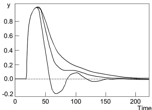
Fig. 6. Load disturbance responses using the Padé approximation:  $\tau_d = 20$ .
