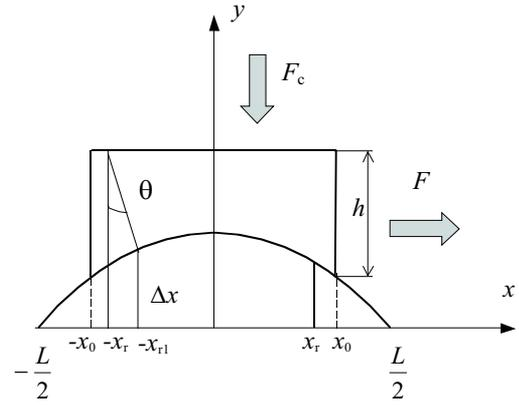
Fig. 3. The contact model between the stator and rotor taking account of shearing deformation
