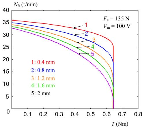
**Fig. 5.** The mechanical characteristics with different thickness of frictional material
