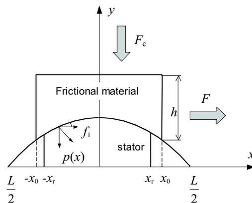
**Fig. 1.** The contact model between the stator and rotor
