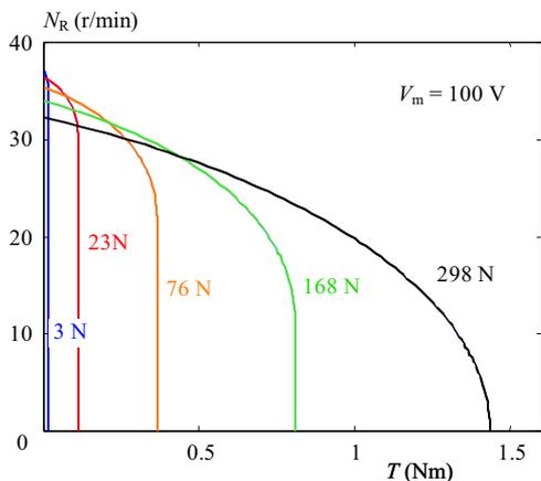
**Fig. 6.** The mechanical characteristics with different preloads
