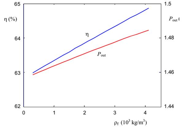
**Fig. 8.** The relationships of maximum efficiency and output power with the density of frictional material
