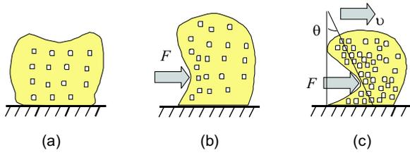
Fig. 2. The sketch of shearing deformation
