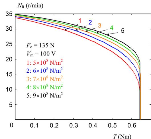
Fig. 4. The mechanical characteristics with different  $E_f$
