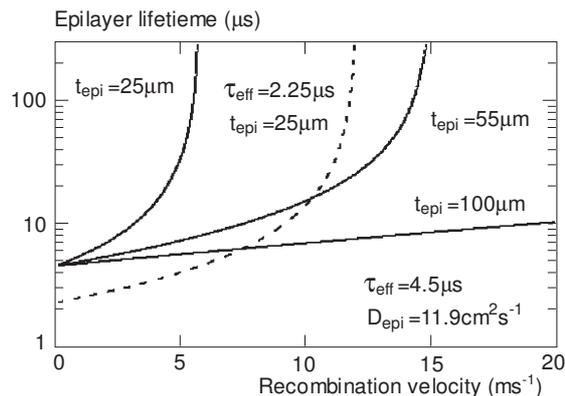
**Fig. 8.** Epitaxial layer lifetime  $\tau_{epi}$  versus recombination velocity  $s_r$  as a function of layer thickness for given effective lifetime. Solid line is solved for  $\tau_{eff} = 4.5 \mu\text{s}$  and dash line for  $\tau_{eff} = 2.25 \mu\text{s}$ .
