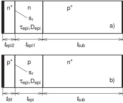
**Fig. 2.** Samples geometry for a.)  $n^+np^+$  and b.)  $p^+pn^+$  structures.
