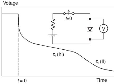
**Fig. 1.** OCVD measurement principle with voltage waveform and schematic (inset).
