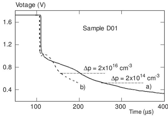
**Fig. 3.** OCVD response of the sample D01 a.) after edge etching and b.) before edge etching. Dash-dot lines denote injection levels of minority carriers.
