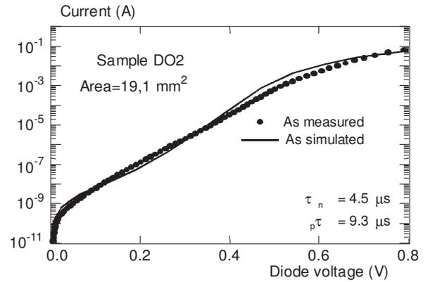
**Fig. 6.** As measured and simulated  $I$ - $V$  characteristic of the sample D02. For simulation,  $\tau_n$  and  $\tau_p$  obtained from OCVD measurement was used with assumption that energy of dominant trap is located at mid-gap  $E_T = E_i$ .
