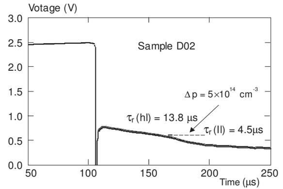
**Fig. 4.** OCVD response of the sample D02. Dash-dot line denotes injection level of minority carriers equal to base doping, *ie* transition from high to low-level injection.
