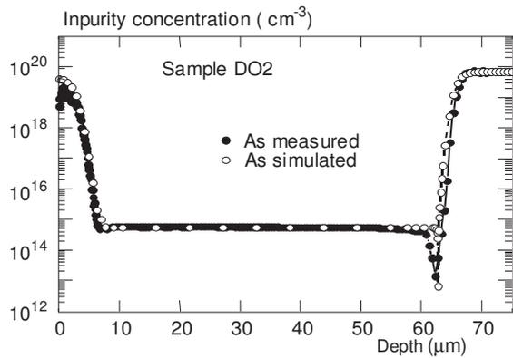
**Fig. 5.** Experimental (spreading resistance profiling) and simulated impurity depth profile of the sample D02.
