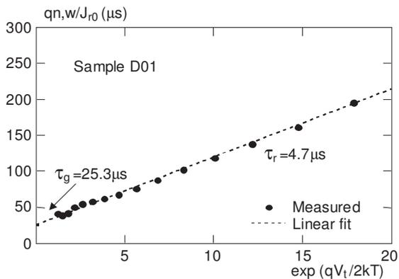
**Fig. 7.** Extraction of recombination and generation lifetime from  $I$ - $V$  and  $C$ - $V$  experimental data according to ref. [10].
