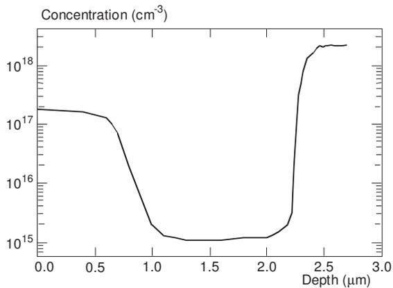
Fig. 3. The profile  $N(x)$  by PCIV method measurement
