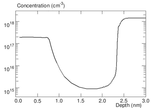
Fig. 4. The  $N(x)$  profile by ECV measured
