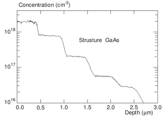
Fig. 2. The  $N(x)$  profile step-like GaAs structure by ECV technique measured
