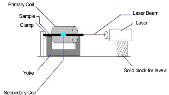
Fig. 2. Diagram of experimental setup
