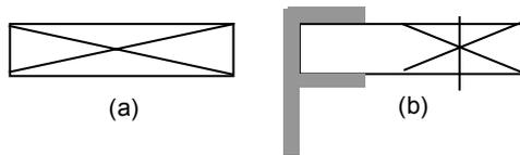
Fig. 1. Resonance condition of the sample with (a) free end and (b) clamped end
