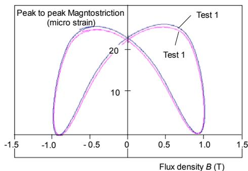
Fig. 6. Magnetostriction,  $\lambda$  vs Flux Density,  $B$  at 2250Hz at  $B_{\max} = 1.0T$
