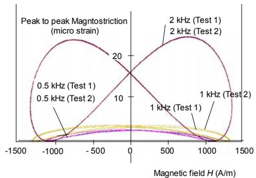
Fig. 5. Magnetostriction,  $\lambda$  vs Magnetic Field,  $H$  at 500Hz, 1000Hz, 2000Hz at  $B_{max} 1.0T$
