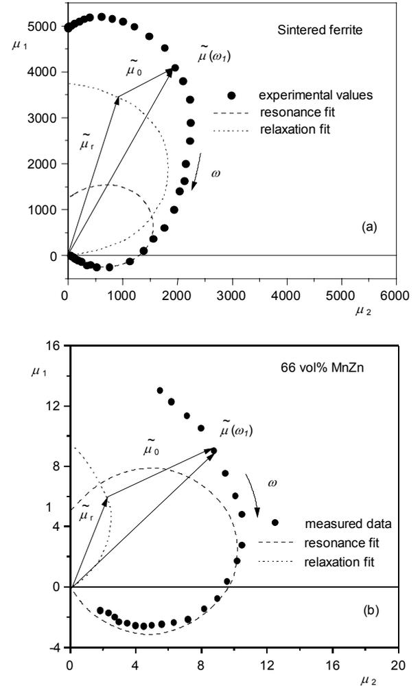
Fig. 2. The complex permeability spectra of sintered MnZn ferrite (a) and of ferrite polymer with  $\kappa_v = 66.0$  vol% MnZn composite.
