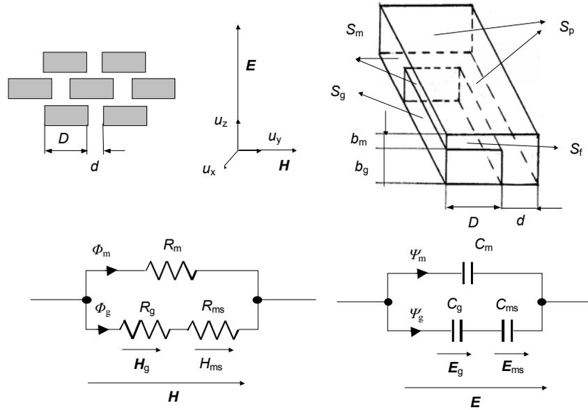
Fig. 1. The model of filler particles structure arrangement in polymer matrix: array of particles and elementary cell of composite (a), models of magnetic and dielectric circuit (b).
