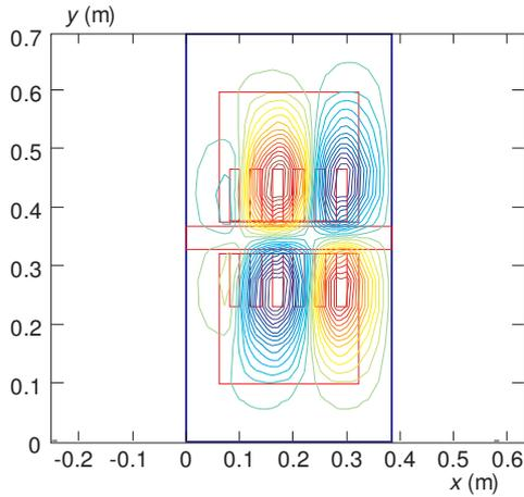
Fig. 5. Magnetic vector potential distribution in the MHD pump
