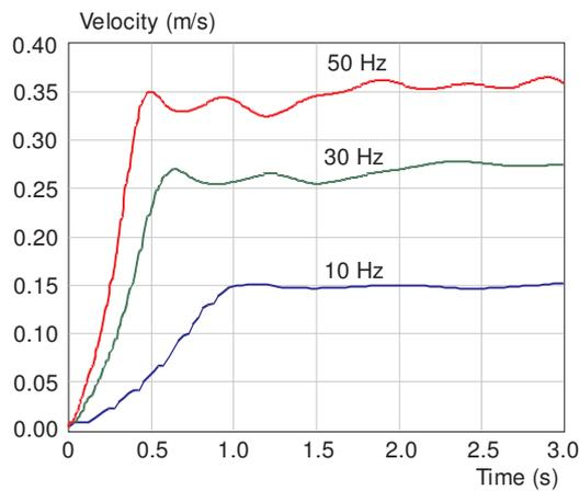
Fig. 9. Velocity in the middle of the channel for several frequencies
