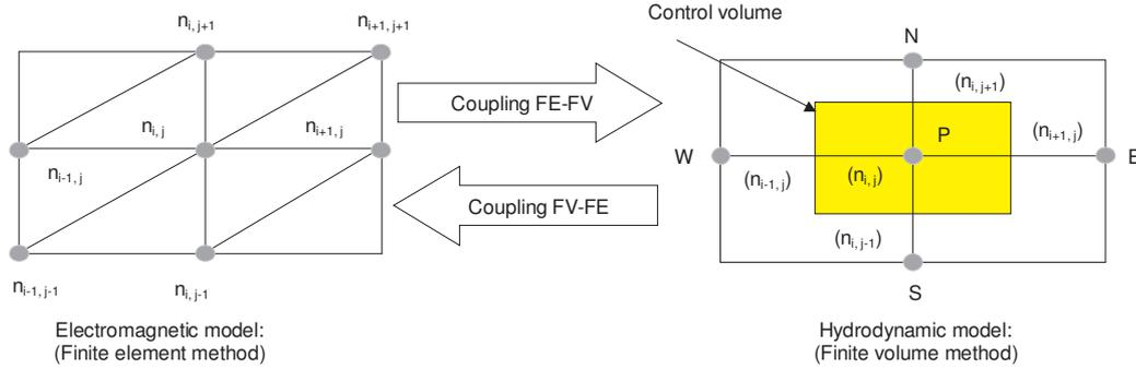
Fig. 3. The adaptation of the nodes for the coupling F.E-F.V
