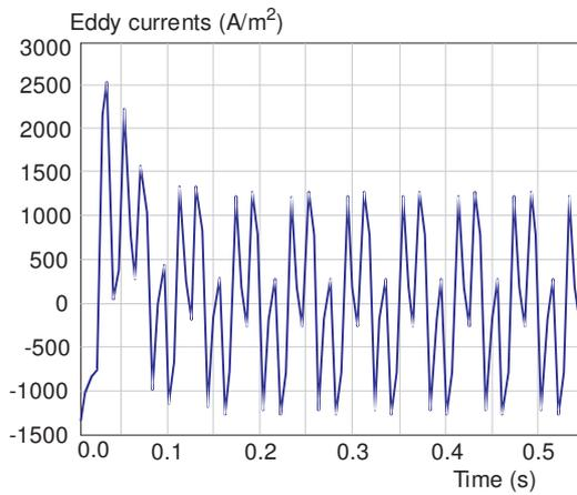
Fig. 7. Eddy currents at the starting for  $f = 50$  Hz
