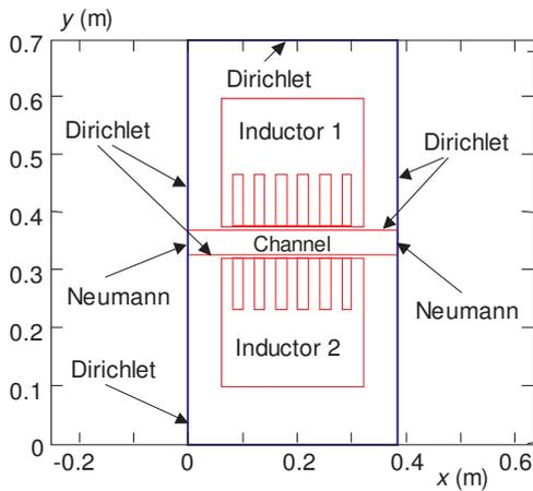
Fig. 2. Schematic view of the MHD pump
