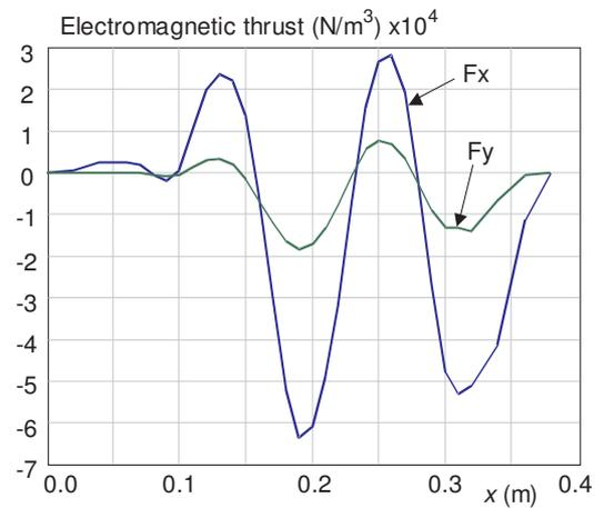
Fig. 8. The electromagnetic thrust for  $f = 50$  Hz
