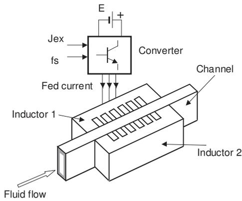
Fig. 1. The prototype of the MHD
