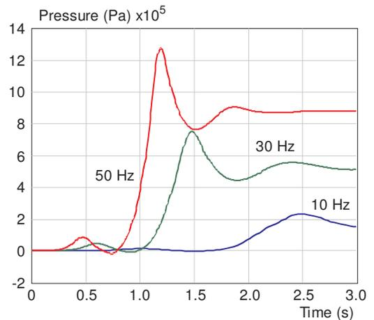
Fig. 10. Pressure in middle of the channel for several frequencies
