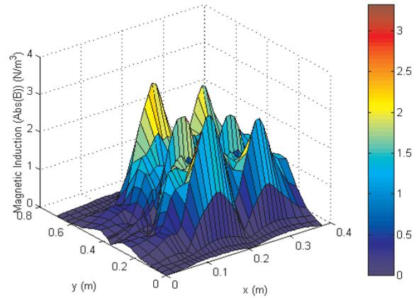
Fig. 6. The magnetic induction in the MHD pump
