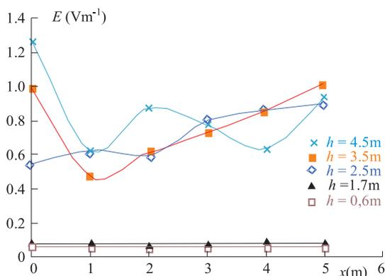
Fig. 5. Intensity of electric field emitted by a HV line of shielded overhead conductors. (Distribution with electrically shielded conductors, see Fig. 11).
