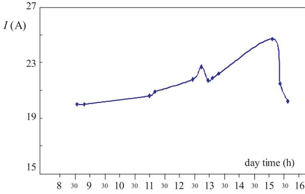
**Fig. 1.** Power off-take from HV line in measuring electric field intensity. The chronological course of the power off-take is not constant.
