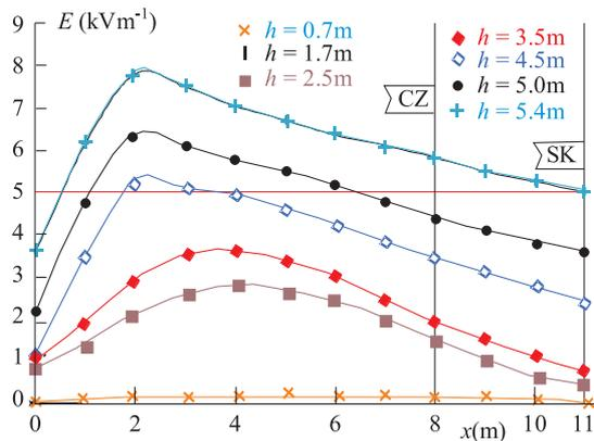
Fig. 3. Electric field intensity emitted by HV line of bare conductors.
