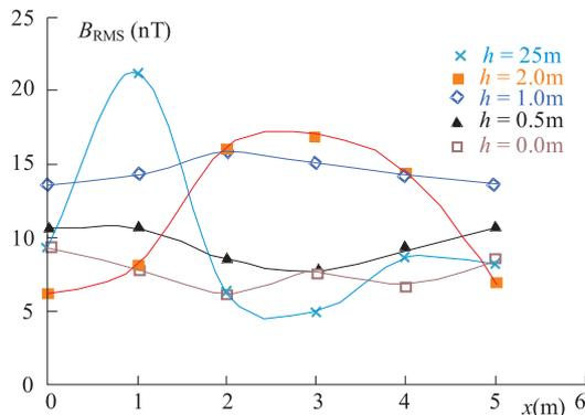
**Fig. 9.** Magnetic flux density due to shielded overhead lines of 22 kV. The detected size of magnetic induction is negligible. The irregular course is given by non-constant power off-take from the distribution net see Fig. 2 — and the shielding of the component  $B$  due to the electric shielding of the energy distribution.
