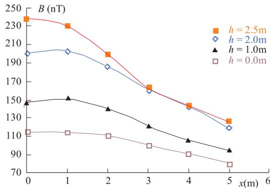
**Fig. 7.** Magnetic flux density due to classical bar of 22 kV HV line
