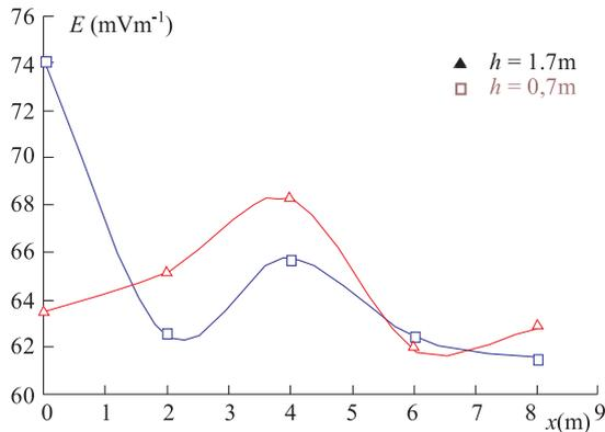
**Fig. 6.** Intensity of electric field  $E$  emitted by a shielded underground HV line of 22 kV/50 Hz for the heights 0.7 m and 1.7 m above ground. The detected size of electric field intensity is negligible. The irregular course is given by non constant power off - take from the distribution net — see Fig. 1 — the shielding of the  $E$  component through the electric shielding of the energy distribution, and by absorption in the soil.
