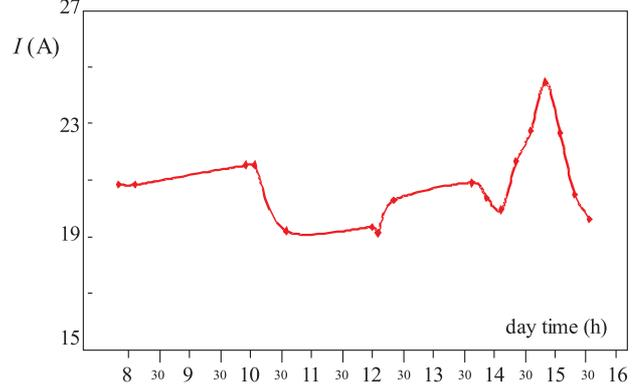
**Fig. 2.** Power off-take from HV line in measuring magnetic flux density. The chronological course of the power off-take is not constant.
