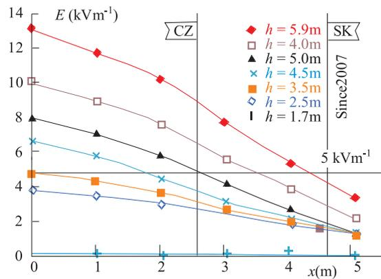
Fig. 4. Intensity of electric field emitted by a HV line of insulated conductors (conductors with basic insulation).
