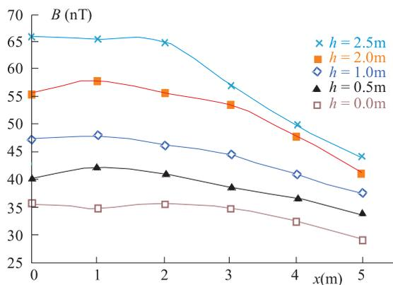
**Fig. 8.** Magnetic flux density due to insulated HV lines of 22 kV. The irregular course is given by non-constant power off-take from the distribution net (see Fig. 2).
