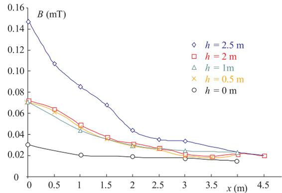
**Fig. 10.** Magnetic flux density emitted by a shielded underground line of 22 kV for heights 0, 1, 2, and 2.5 m above ground. The detected size of magnetic induction is higher than results presented in Fig.7 to Fig.9. The irregular course is given by non-constant power off-take from the distribution net see Fig. 2 — and the shielding of the  $B$  component due to the electric shielding of the energy distribution and by absorption in the soil.
