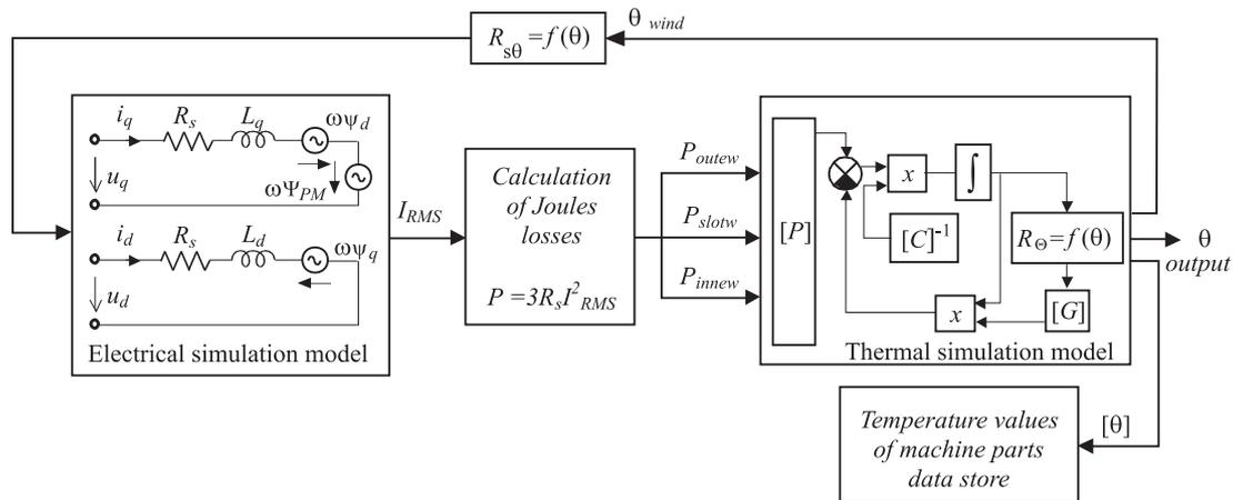
Fig. 5. Block diagram of the simulation model consisting of electrical and thermal model.
