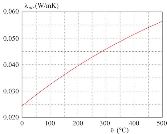
Fig. 3. Thermal conductivity of the air versus temperature according to [6].
