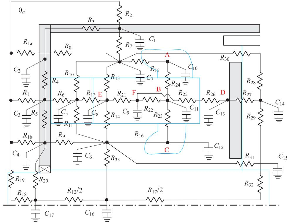
Fig. 2. Simplified thermal network of analyzed AFPM.
