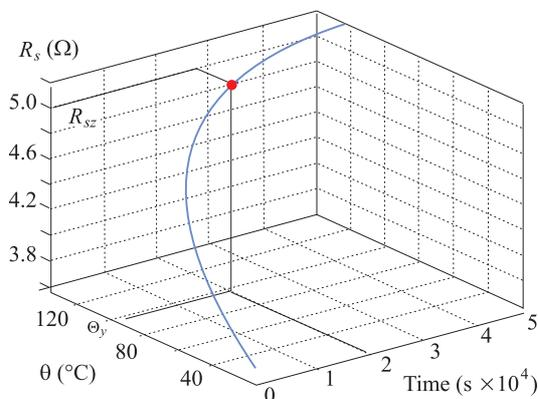
Fig. 6. The thermal change of stator resistance in time.
