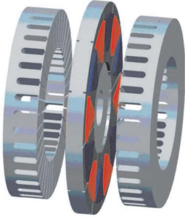
**Fig. 4.** Structure of AFPM, in which one rotor is located between two stators.
