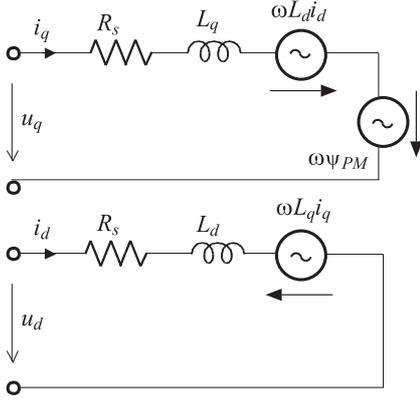
Fig. 1. Equivalent circuit of AFPM in  $d$  and  $q$  axis.
