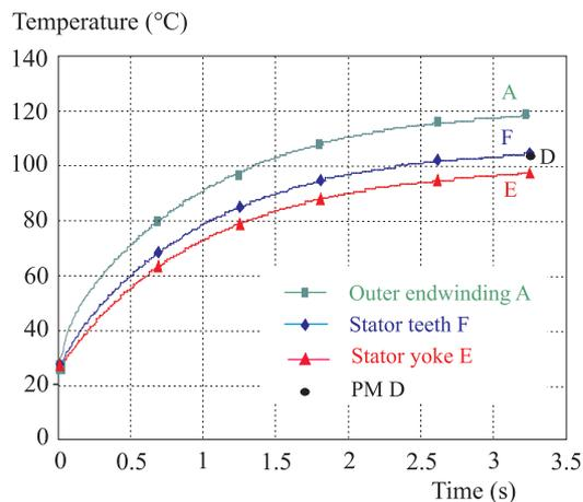
Fig. 9. Measured temperatures in nodes marked by letters *A*, *D*, *E* and *F* in Fig.2.
