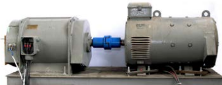
Fig. 4. The electromachine unit for investigations of a synchronous generator
