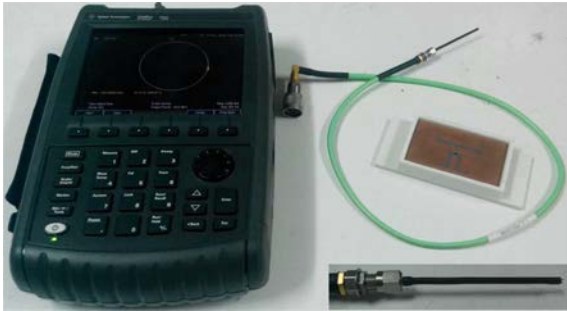
Fig. 5. Setup for measuring the antenna impedance
