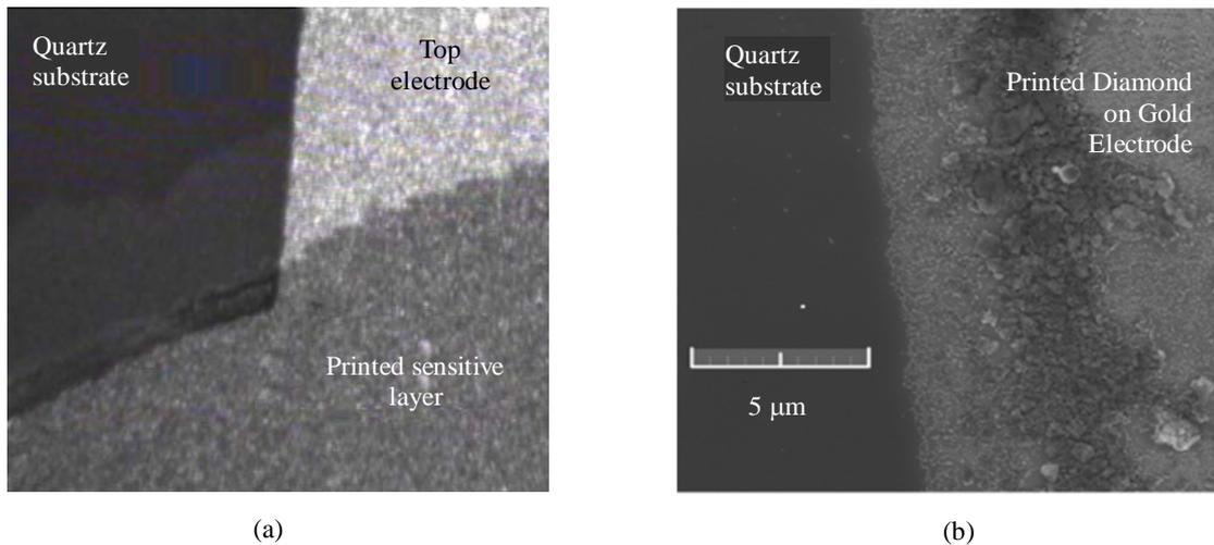
**Fig. 2.** (a) — Optical micrograph of the printed diamond-ethylene glycol solution on the quartz substrate before evaporation, (b) — SEM image of printed diamond powder
