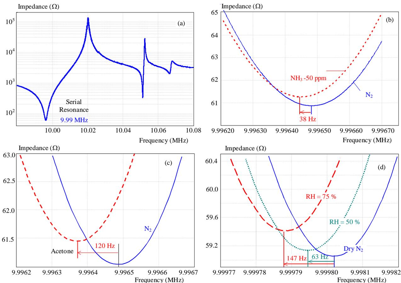
**Fig. 4.** (a) — Impedance characteristics of the sensor under test with a serial/parallel resonance peak and spurious modes; detail of shift in serial resonance after exposure to (b) — 50 ppm of ammonia, (c) 1% of acetone vapour, (d) — change in relative humidity from 0% RH to 75% RH
