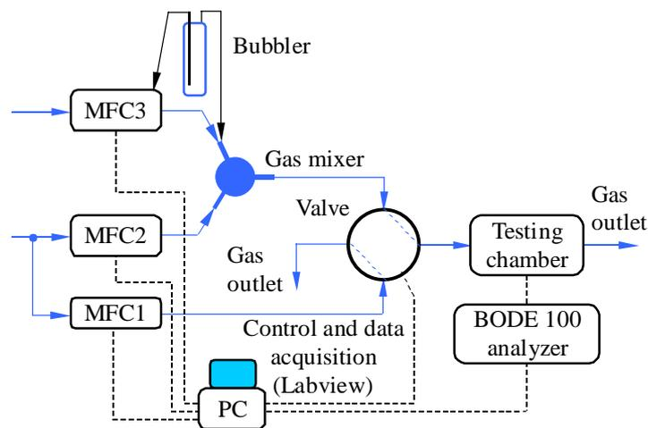
**Fig. 3.** Schematic drawing of the apparatus for sensor characterization
