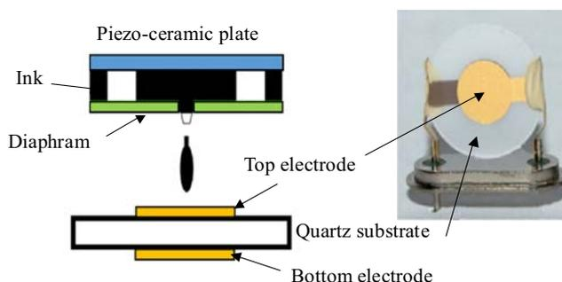
**Fig. 1.** Structure of the QCM sensor with a schematic drawing of ink-jet printing of a sensitive layer and a real sample mounted in HC-51/U package
