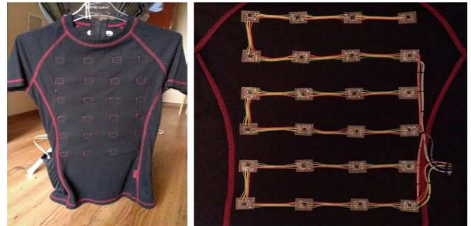
Fig. 6. Biometric T-shirt and inside sensors detail, right
