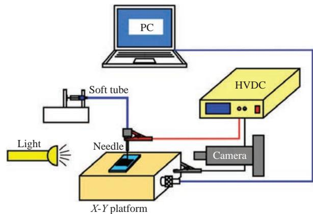
**Fig. 1.** Schematic of the printing apparatus
