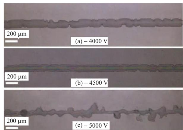
Fig. 3. Micrographs showing the printed patterns at different applied voltages
