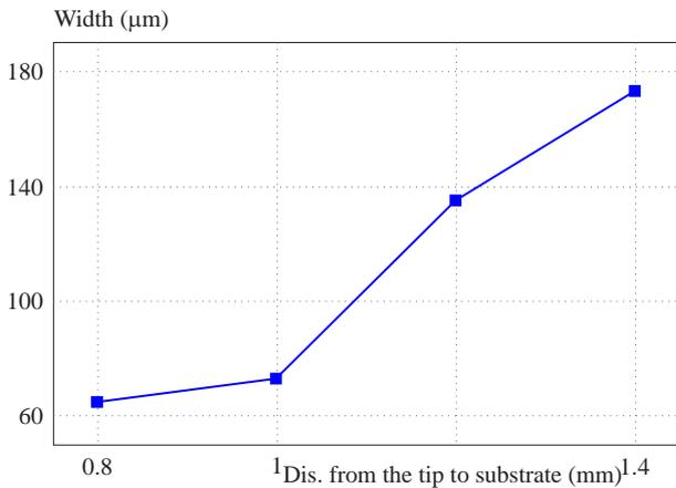
Fig. 8. The effect of needle-substrate distance on the printed line width
