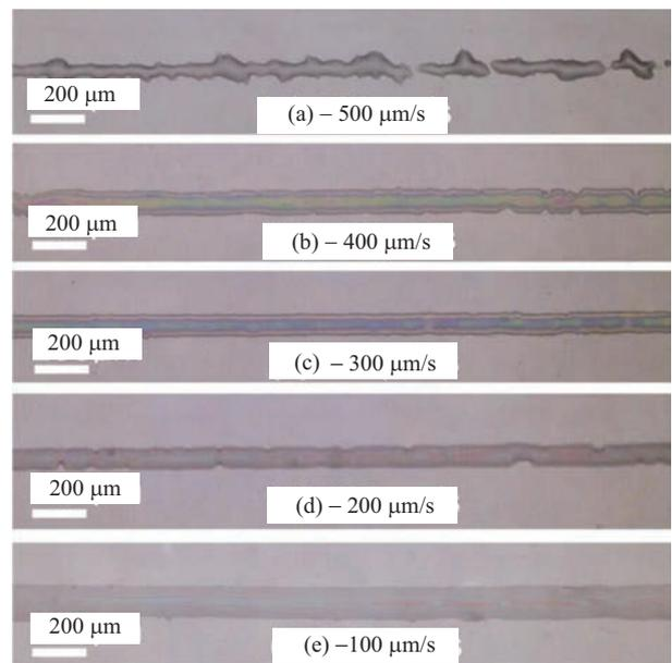
Fig. 10. Micrographs showing the printed patterns at different platform moving speed
