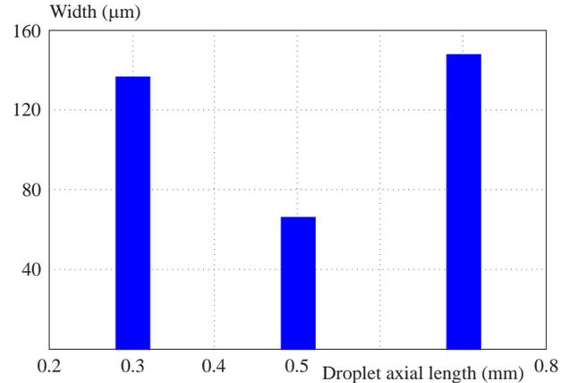
**Fig. 5.** The influence of droplet axial length on the width of printed lines
