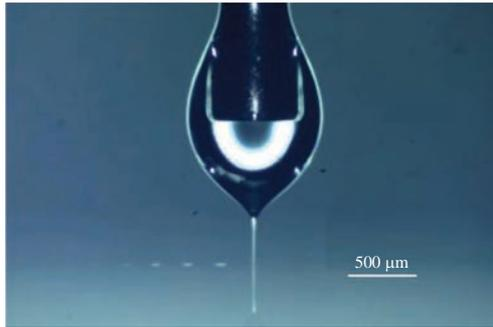
Fig. 2. Intermittent cone jet of silicone oil
