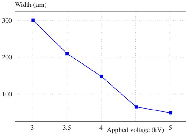
**Fig. 4.** The relationship between the applied voltage and the width of printed lines
