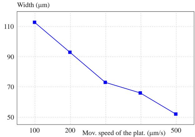
Fig. 9. The effect of moving speed of platform on the printed line width
