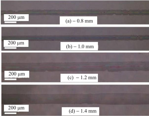
Fig. 7. Micrographs showing the printed patterns at different needle-substrate distance
