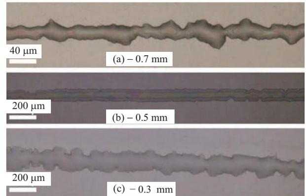
**Fig. 6.** Micrographs showing the printed patterns at different axial lengths
