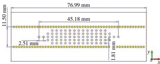
Fig. 3. The simulation model of the phase shifter based on the SIW technology with an initial density of the array holes
