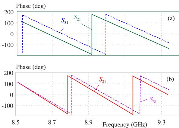
Fig. 11. Simulated phases of the reference test circuit (a) – without phase shifter, and (b) – the test circuit with the phase shifters
