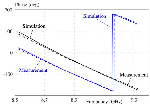
Fig. 8. Frequency response of phase shift: simulation (solid), measurement (dashed)
