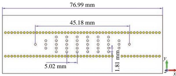
Fig. 5. The simulation model of the phase shifter - layout of the air holes in  $xy$  plane
