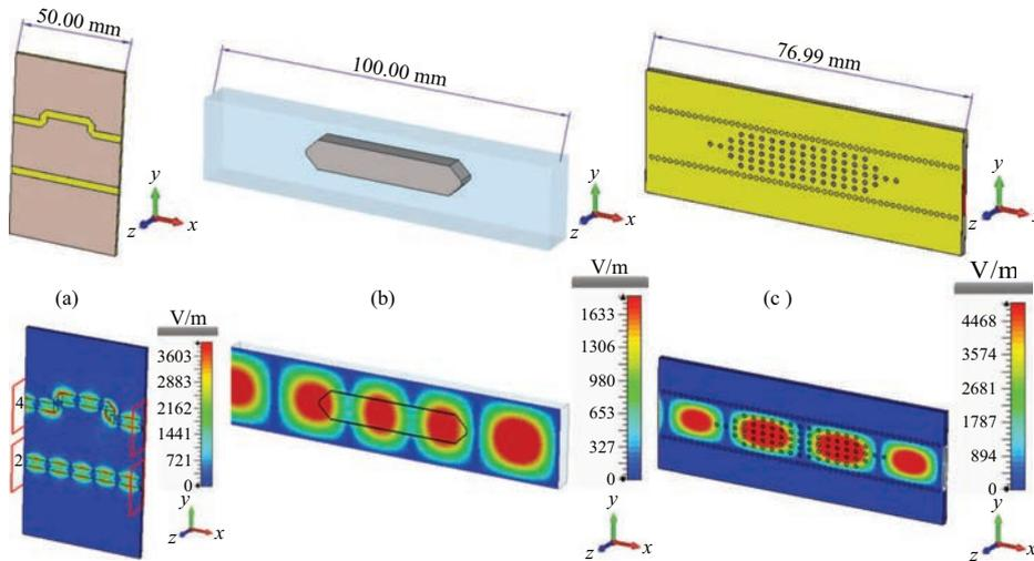
Fig. 1. An example of phase shifters: (a) – microstrip line, (b) – metallic waveguide, and (c) – SIW technology, simulated at 8.925 GHz
