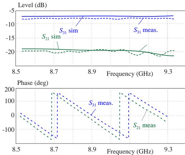
**Fig. 14.** Frequency response of the test circuits: top – simulated and measured coefficients of the transmission, bottom – measured phase
