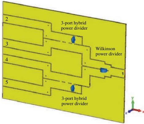
Fig. 9. The simulation model of the reference test circuit
