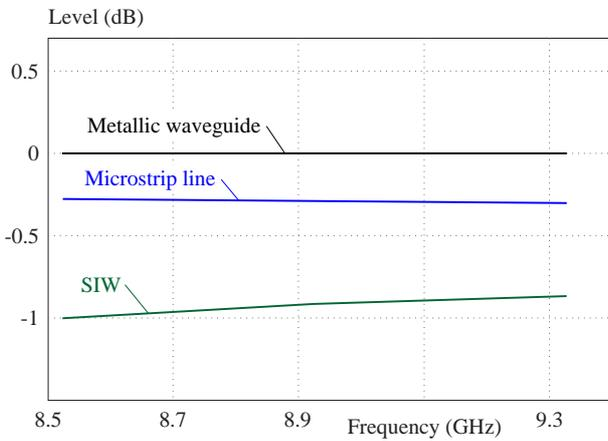
Fig. 2. Frequency response of transmission coefficient: metallic waveguide (black), microstrip line (blue), SIW (green)
