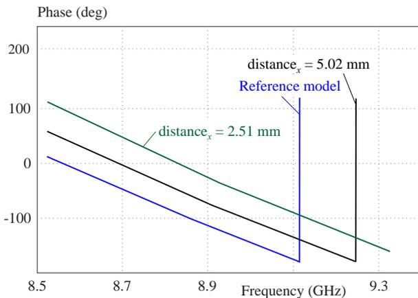
Fig. 6. Simulated frequency response of phase shift for different distance of vias:  $\Delta x = 5.02$  mm (black),  $\Delta x = 2.51$  mm (green), reference (blue)
