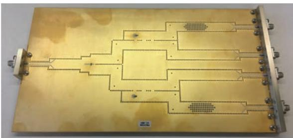
Fig. 12. Fabricated prototype of the test circuit
