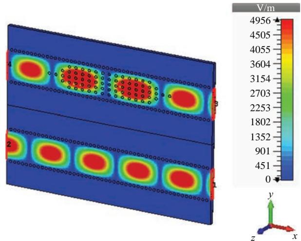
Fig. 4. The E-field simulation the phase shifter based on the SIW technology
