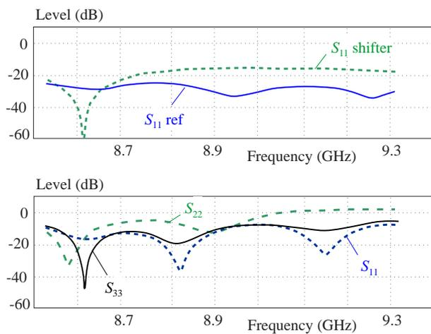
**Fig. 15.** Measured reflection coefficients: (top) – reference waveguide and phase shifter, (bottom) – test circuits
