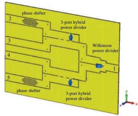
Fig. 10. The simulation model of the test circuit
