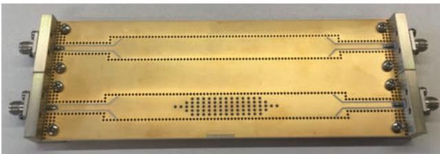
Fig. 7. Fabricated prototype of the phase shifter (down) and the reference waveguide (up)
