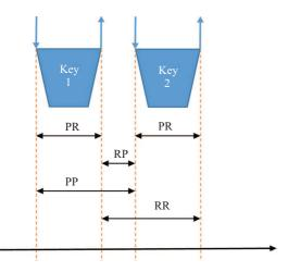
Fig. 1. Representation of keystroke dynamics time information data with press (P) and release (R) events of the keys
