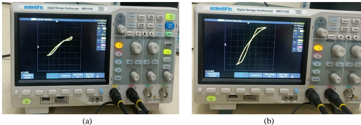
Fig. 11. Transient v - i curves of the LM13700-based inverse memristor emulator (given in Fig. 10) on the DSO screen: (a) for 15 kHz, (b) for 20 kHz
