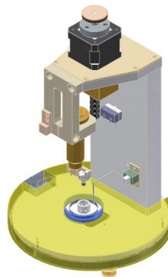
Fig. 1. Model of the device for etching with a mechanical holder of the tip which is driven by a precise micro-stepper motor [8]
