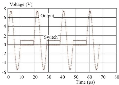
Fig. 4. Simulation of the voltage waveform for the  $LC$  resonant circuit.
