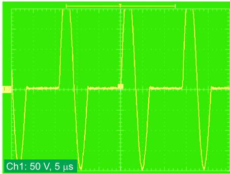
**Fig. 13.** Actual waveform (1 resonant cycle when switch is OFF).
