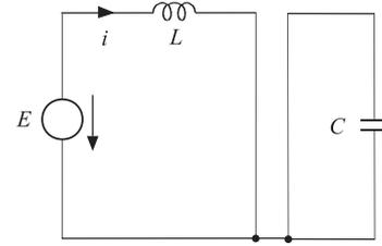
Fig. 6. Equivalent circuit when switch is ON.
