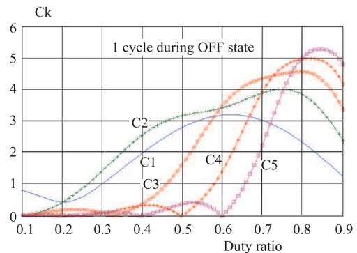
Fig. 9. Relations of amplitudes of harmonic waves with driving duty ratio (1 resonant cycle when switch is OFF)
