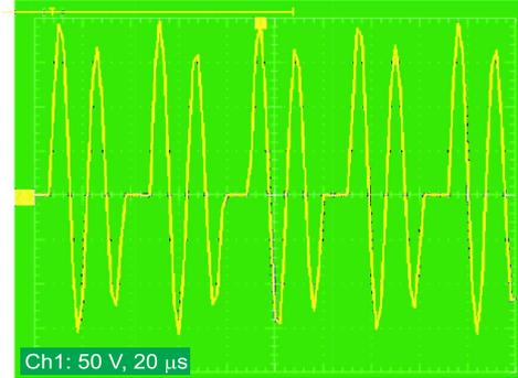
**Fig. 14.** Actual waveform (2 resonant cycles when switch is OFF).
