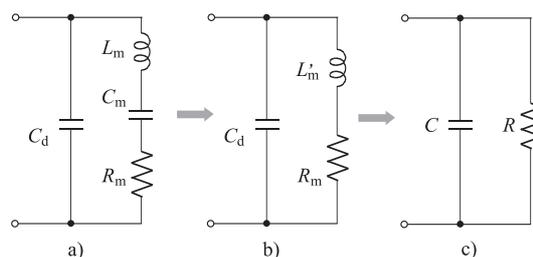
Fig. 2. Transformation of USM equivalent circuit.
