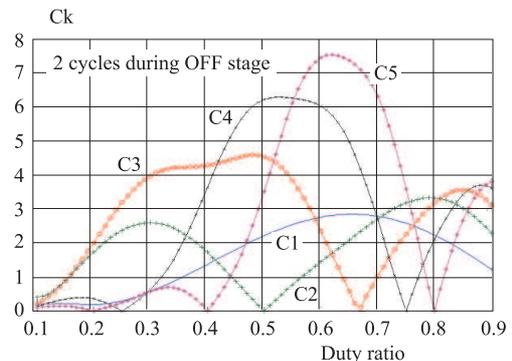
Fig. 10. Relations of amplitudes of harmonic waves with driving duty ratio (2 resonant cycles when switch is OFF).
