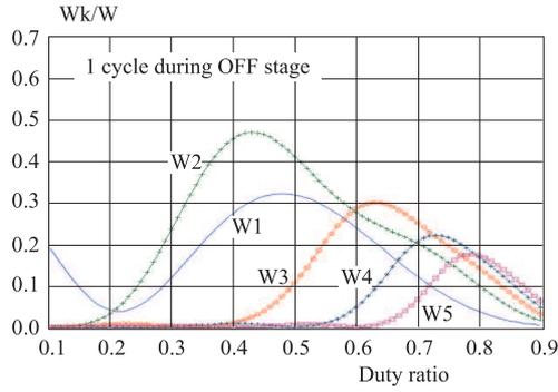
**Fig. 11.** Relations of energy efficiency of harmonic waves with driving duty ratio (1 resonant cycle when switch is OFF).
