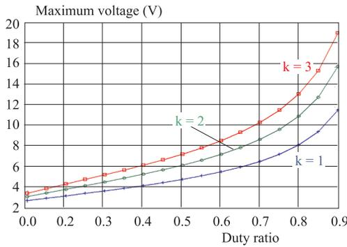
Fig. 8. Maximum voltage under different resonant cycles.
