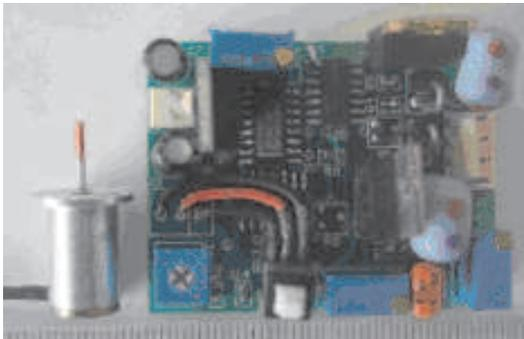
**Fig. 15.** The driver and the ultrasonic motor.
