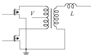
Fig. 1. Push-pull transformer circuit for USM.
