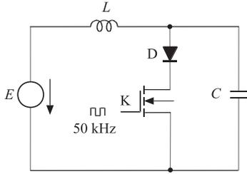
Fig. 3. The non-transformer driving circuit for USM.
