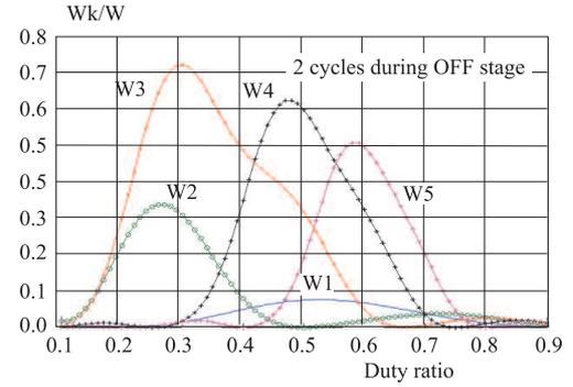
**Fig. 12.** Relations of energy efficiency of harmonic waves with driving duty ratio (2 resonant cycles when switch is OFF).
