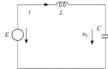
Fig. 7. Equivalent circuit when switch is OFF.
