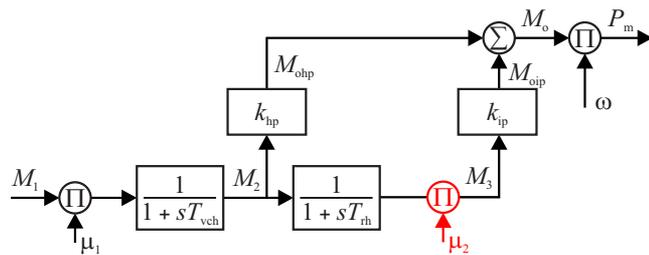
Fig. 2. The model of the two cases steam turbine with the intermediate pressure intercept valve
