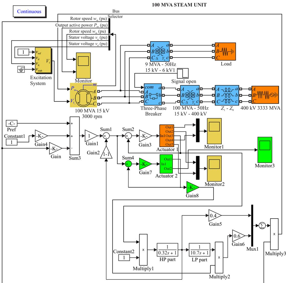
Fig. 3. The model of the turbogenerator connected to the grid
