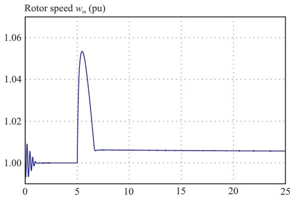
Fig. 4. Output speed with IPIV
