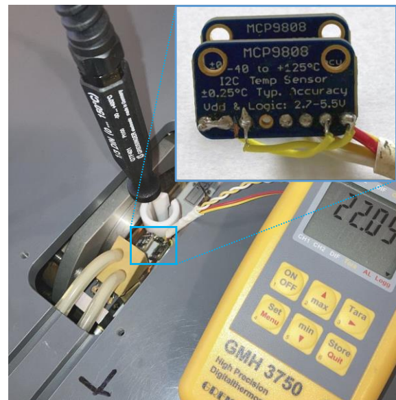
Fig. 6. Documentary photo of evaluated temperature sensors MCP9808 during comparative measurement by the high-precision thermometer GMH 3750 inside the Minispec pc 100 device
