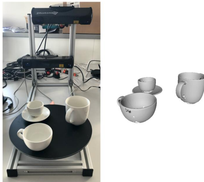
Fig. 1. Rotary table and 3D model of the scene
