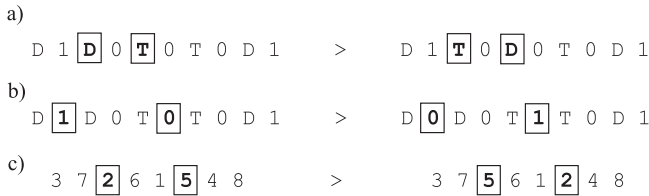
Fig. 7. Mutation operator: a) only flip-flop types are changed, b) inverter presences are changed, and c) pattern orders and test bit streams order are changed.
