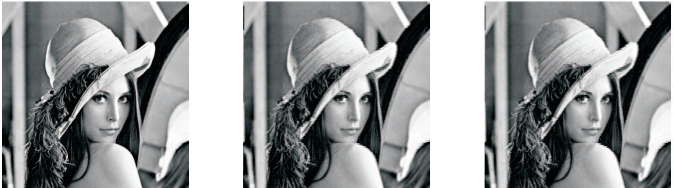
Fig. 2. The Lena picture a) original, b) used SFC (block 4 \times 4 ) scanned with normal raster and DPCM with 2 bits/pixel and constant quantization levels, c) DPCM with 2 bits/pixel and constant quantization levels.
