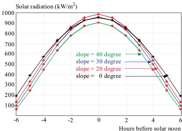
**Fig. 3.** Hourly clear-sky solar radiation (beam + diffuse), latitude = 40N, solid lines = simulations results, asterisks = measured data
