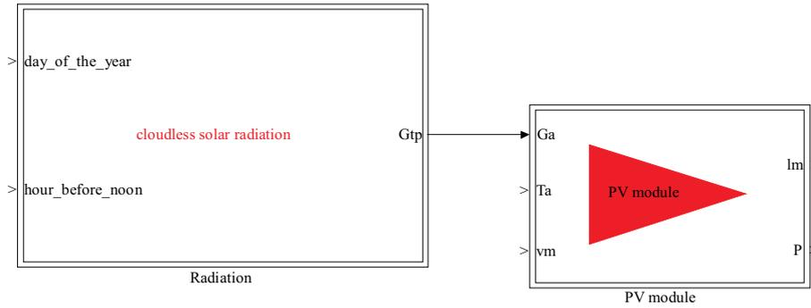
Fig. 2. Matlab/Simulink structure for PV module
