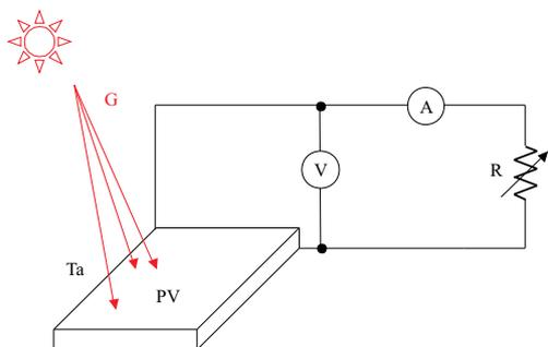
**Fig. 4.** Experiment set up
