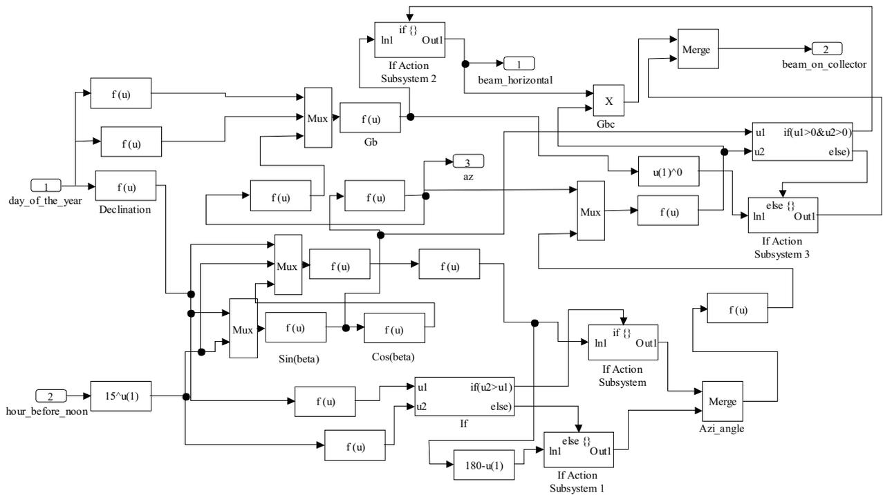
Fig. 9. Matlab/Simulink structure of the beam radiation
