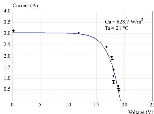
**Fig. 6.** Experimental and predicted data of  $(V, I)$  for PV module; day = 132 (12/05) at 10:00 am; slope = 5 degree
