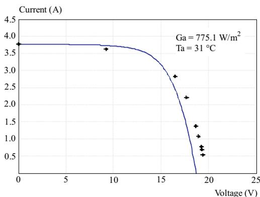
**Fig. 5.** Experimental and predicted data of  $(V, I)$  for PV module; day = 129 (09/05) at noon; slope = 5 degree
