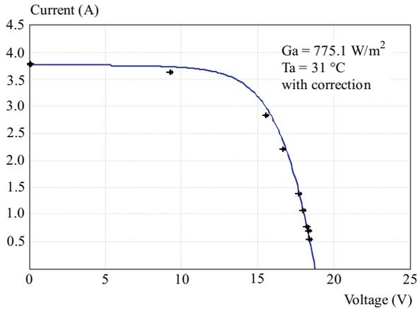
Fig. 7. Experimental and predicted data of  $(V, I)$  for PV module; day = 129 (09/05) at noon; slope = 5 degree
