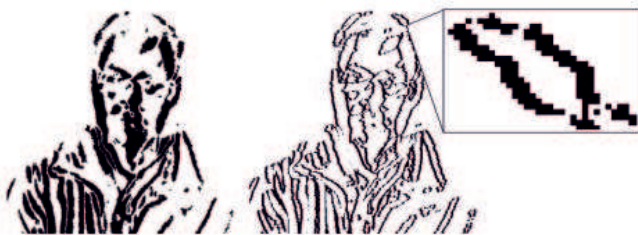
Fig. 6. Detected motion as the input data for edge detection (left), the result of the detected edges by a standard Laplace edge detector (right)
