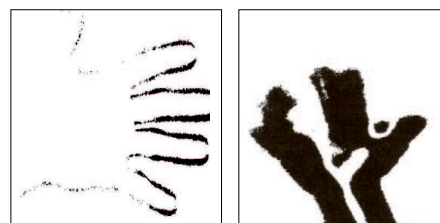
Fig. 2. Motion detection using the low threshold (left), motion detection using a slow algorithm (right)
