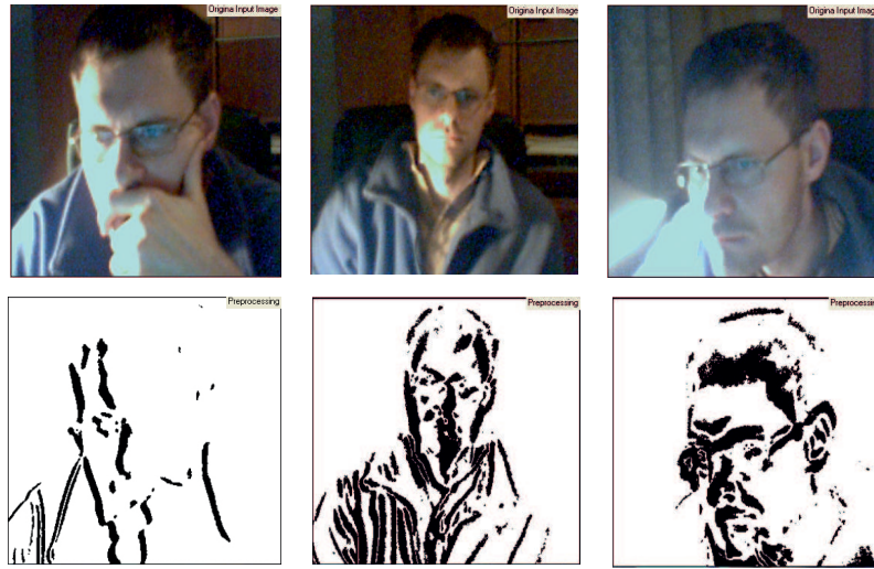
Fig. 5. Motion input in the row, the result of motion detection at the bottom. Slow motion in the left column, faster motion in the middle column and motion under direct strong light in the right column
