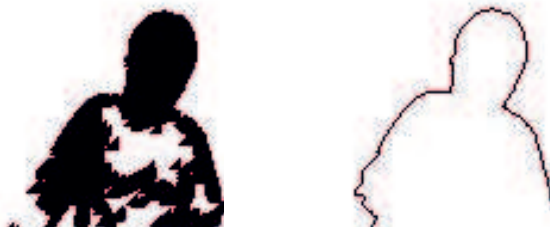
Fig. 15. Motion detection with multi-erosion (left), detected longest edge (right)
