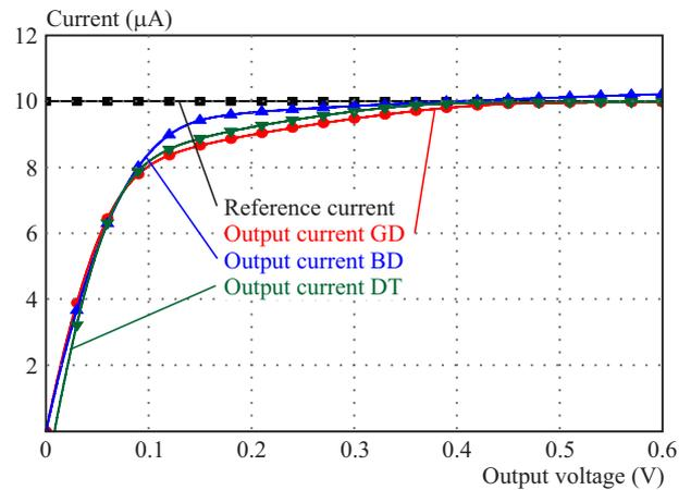
Fig. 20. Output characteristics of cascode CMs
