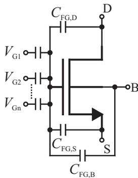
Fig. 3. Parasitic capacities of FGMOS transistor
