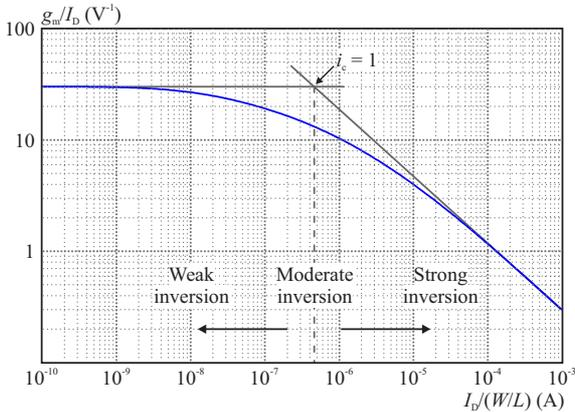
Fig. 6. Parameter  $g_m/I_D$  versus the normalized drain current
