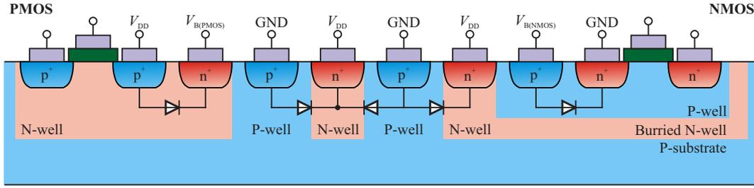
Fig. 12. Cross-section of CMOS structure with guard rings
