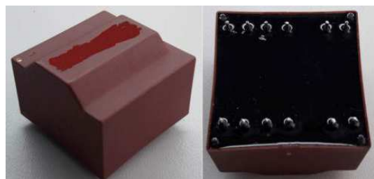
Fig. 4. Photo of the transformer T2-3
