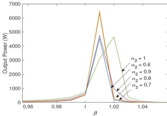
Fig. 15. Output power versus  $\beta_{1,2}$  when  $0.5 < \alpha_2 \leq 1$  at  $\alpha_1 = 1$
