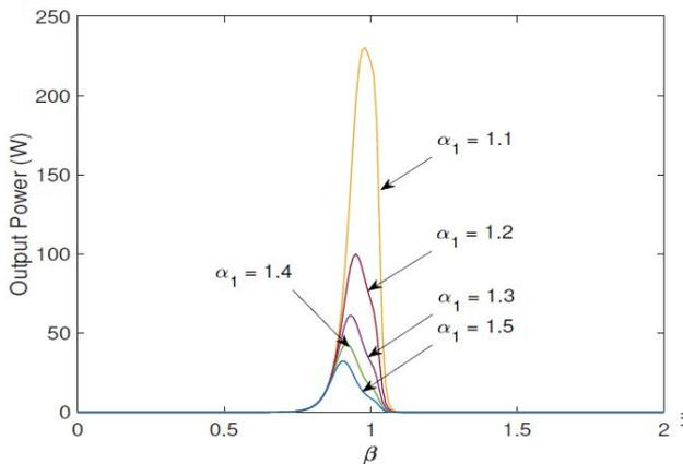
Fig. 11. Output power versus  $\beta_{1,2}$  when  $1 < \alpha_1 \leq 1.5$  at  $\alpha_2 = 1.2$
