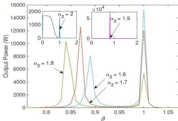
Fig. 17. Output power versus  $\beta_{1,2}$  when  $1.5 < \alpha_2 \leq 2$  at  $\alpha_1 = 1$
