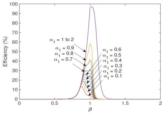
Fig. 13. Efficiency versus  $\beta_{1,2}$  when  $0 < \alpha_1 \leq 2$  and  $\alpha_2 = 1.2$
