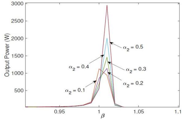
Fig. 14. Output power versus  $\beta_{1,2}$  when  $0 < \alpha_2 \leq 0.5$  at  $\alpha_1 = 1$
