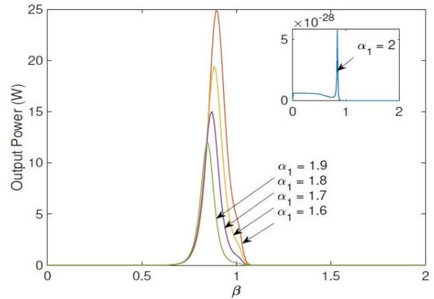
Fig. 12. Output power versus  $\beta_{1,2}$  when  $1.5 < \alpha_1 \leq 2$  at  $\alpha_2 = 1.2$
