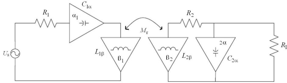
Fig. 1. Equivalent circuit of series-parallel wireless power transfer
