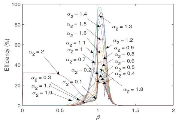
Fig. 18. Efficiency versus  $\beta_{1,2}$  when  $0 < \alpha_2 \leq 2$  at  $\alpha_1 = 1$
