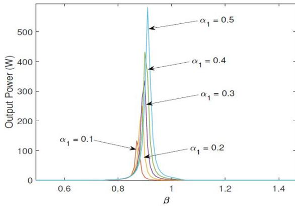
Fig. 9. Output power versus  $\beta_{1,2}$  when  $0 < \alpha_1 \leq 0.5$  at  $\alpha_2 = 1.2$
