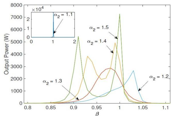
Fig. 16. Output power versus  $\beta_{1,2}$  when  $1 < \alpha_2 \leq 1.5$  at  $\alpha_1 = 1$
