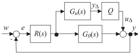
Fig. 4. Standard feedback configuration with additive affine type uncertainty
