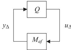
Fig. 5.  $M_{af}$ - $Q$  structure for the additive affine type uncertainty
