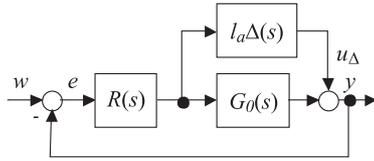
Fig. 2. Standard feedback configuration with additive unstructured uncertainty
