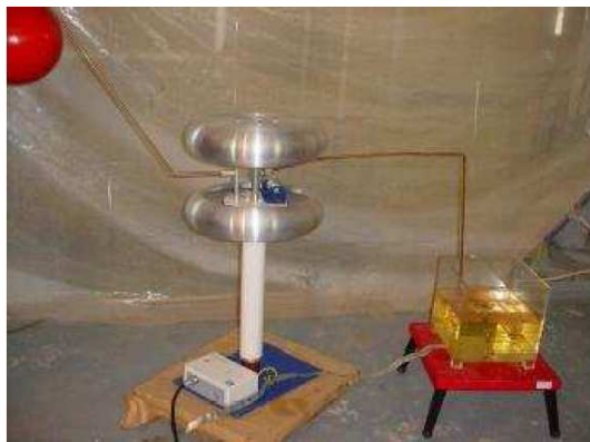
Fig. 3. Photo of the test cell filled with transformer oil, connecting to the coupling capacitor, quadripole and the output of the main transformer
