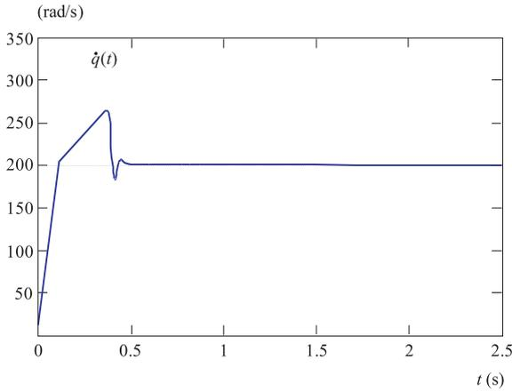
Fig. 9. satPI control + AW: velocity  $\dot{q}(t)$
