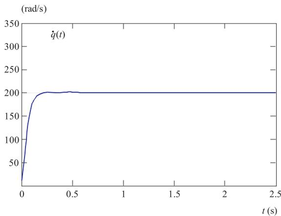
Fig. 7. PI control + AW: velocity  $\dot{q}(t)$ .
