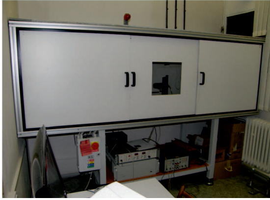
Fig. 2. The enclosed radiation leak protected bench top x-ray imaging system
