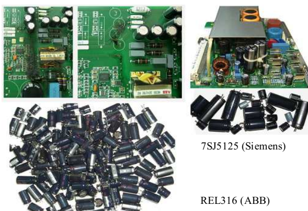
Fig. 2. Faulty DPR switched-mode power supplies of different types with damaged electrolytic capacitors, left figure shows taints in printed circuit boards from electrolyte leakag.
