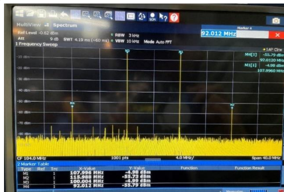
Fig. 11. Measured intermodulation components of two-tone testing
