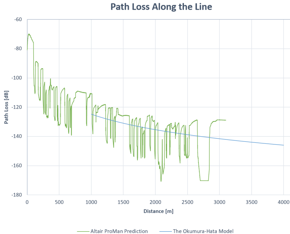
Fig. 17. Comparison of calculated median path loss: Altair ProMan versus Okumura-Hata Model
