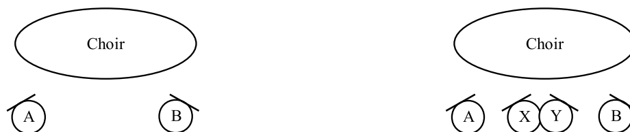
Fig. 1. On the left – AB stereo microphone technique with 30^\circ to 40^\circ sideways-facing, on the right – AB and XY technique combination
