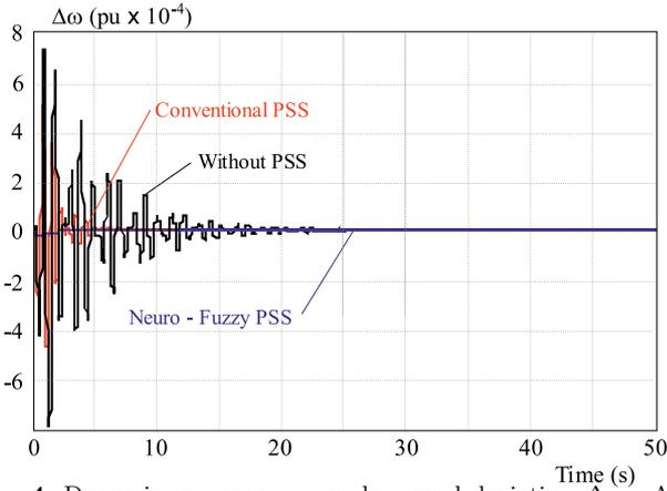
Fig. 4. Dynamic response — angular speed deviation  $\Delta\omega$ , Area 1, for  $P=0.8$  pu,  $Q=0.9$  pu, step torque disturbance = 0.005 pu
