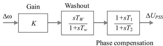
Fig. 2. Structure of Conventional lead-lag PSS (CPSS)
