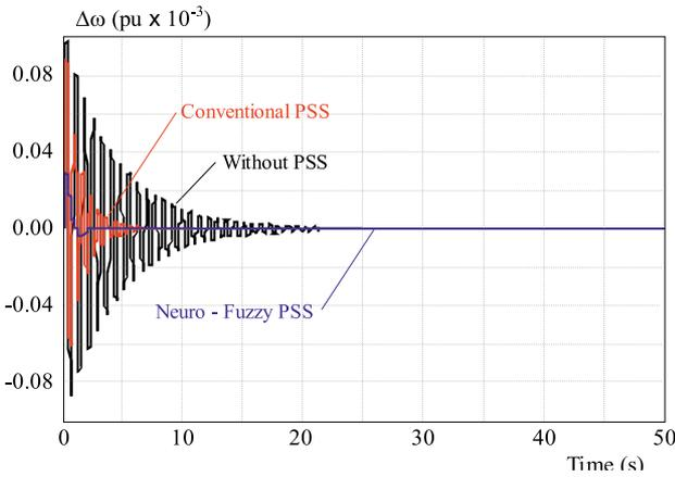
Fig. 6. Dynamic response — angular speed deviation  $\Delta\omega$ , Area 2, for  $P=0.8$  pu,  $Q=0.9$  pu, step torque disturbance = 0.005 pu
