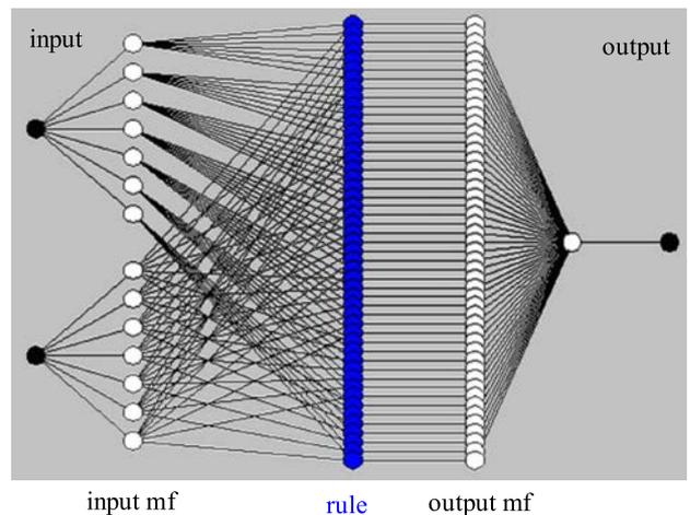
Fig. 3. Structure of proposed ANFIS for the power system under study
