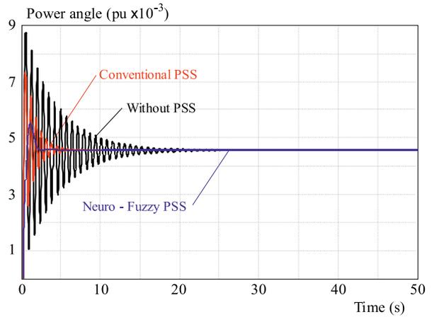
Fig. 7. Dynamic response — power angle, Area 2, for  $P=0.8$  pu,  $Q=0.9$  pu, step torque disturbance = 0.005 pu
