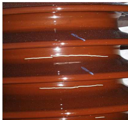
Fig. 1. Crack in the body of insulator
