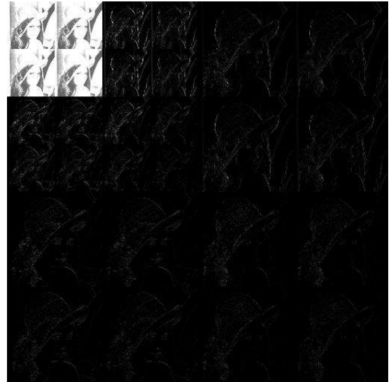
Fig. 16. Two level DMWT of Lena image implemented by 4CH single filters bank
