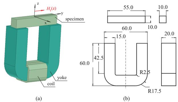
Fig. 2. Magnetic circuit: (a) – geometry, (b) – dimensions
