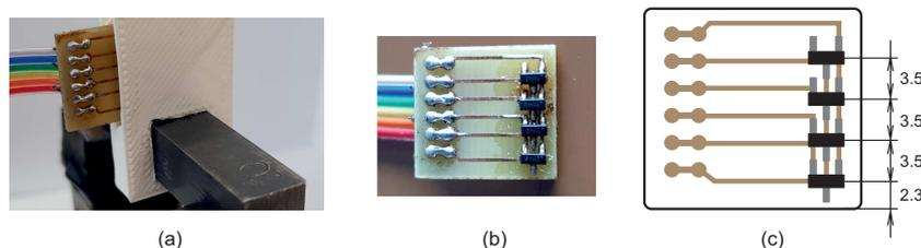
Fig. 6. Sensor: (a) – position on the sample, (b) – detail of the sensor board, and (c) – layout drawing with dimensions
