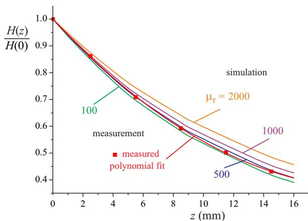
Fig. 5. Dependence of normalised magnetic field intensity on height above sample surface
