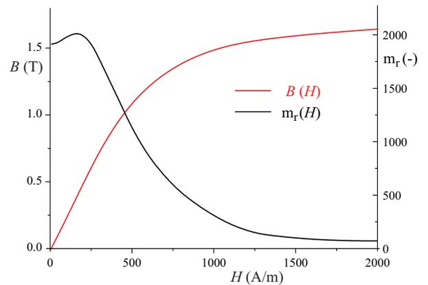
Fig. 4. Initial magnetization path and the dependence of static permeability of steel 12040
