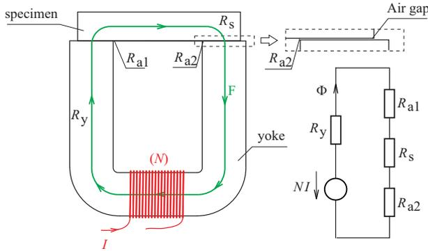
Fig. 3. Model of the magnetic circuit
