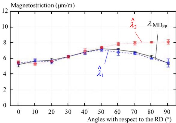
**Fig. 6.** Comparison of  $\lambda_{MDPP}$  measured in Epstein and disc samples of the 0.35 mm thick NO steel
