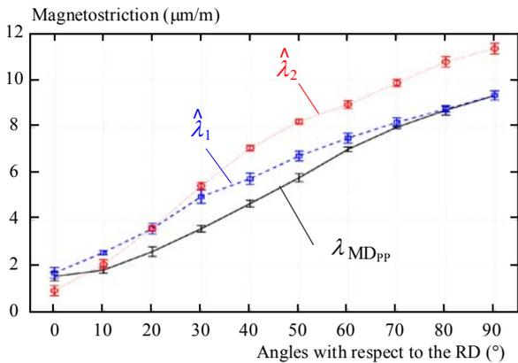
**Fig. 5.**  $\lambda_{MDPP}$ ,  $\hat{\lambda}_1$  and  $-\hat{\lambda}_2$  of the 0.50 mm thick disc sample at 1.50 T versus  $\theta$
