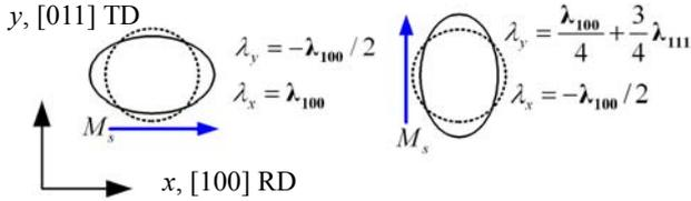
**Fig. 8.** Schematic diagram of magnetostriction components calculated from a single crystal of a Goss-textured GO steel (bar domains) at the demagnetised state and magnetisation along the TD
