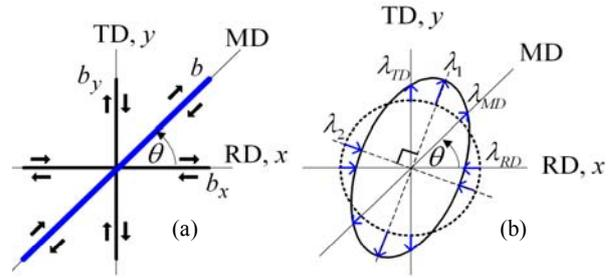
**Fig. 2.** (a) -Vector depicting alternating magnetisation applied to disc samples, (b) - Illustration of magnetostriction components in disc samples
