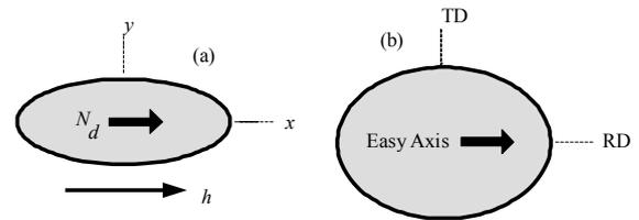
**Fig. 9.** (a) - Demagnetisation factor in an ellipsoid of rotation [12], (b) - Equivalent shape of the 0.50 mm disc sample due to the magnetic anisotropy
