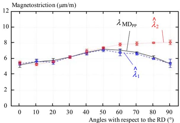
**Fig. 4.**  $\lambda_{MDpp}$ ,  $\hat{\lambda}_1$  and  $-\hat{\lambda}_2$  of the 0.35 mm thick disc sample at 1.50 T versus  $\theta$
