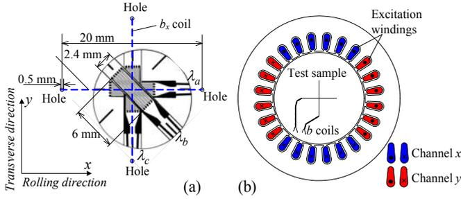
**Fig. 1.** (a) - Locations of rosette resistance strain gauges and orthogonal  $b$  coils at the centre of a disc sample, (b) -Schematic diagram of a disc sample placed in a magnetising yoke of the 2D magnetisation system
