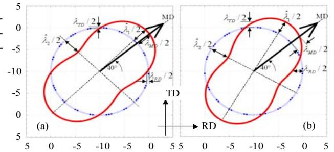
**Fig.3.** Magnetostriction components of (a) the 0.35 mm thick disc sample and (b) the 0.50 mm thick disc sample both at 1.70 T and  $\theta=40^\circ$
