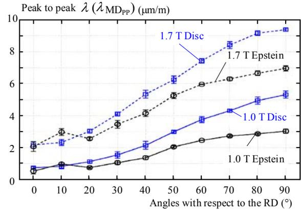
**Fig. 7.** Comparison of  $\lambda_{MDPP}$  measured in Epstein and disc samples of the 0.50 mm thick NO steel
