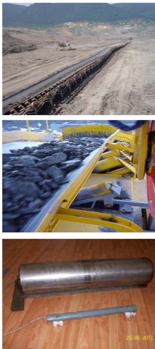
Fig. 1. ( a) - Conveyor excavator, ( b) - measuring roller with gravity positioning beneath the conveyor belt, ( c) - roller and induction sensor
