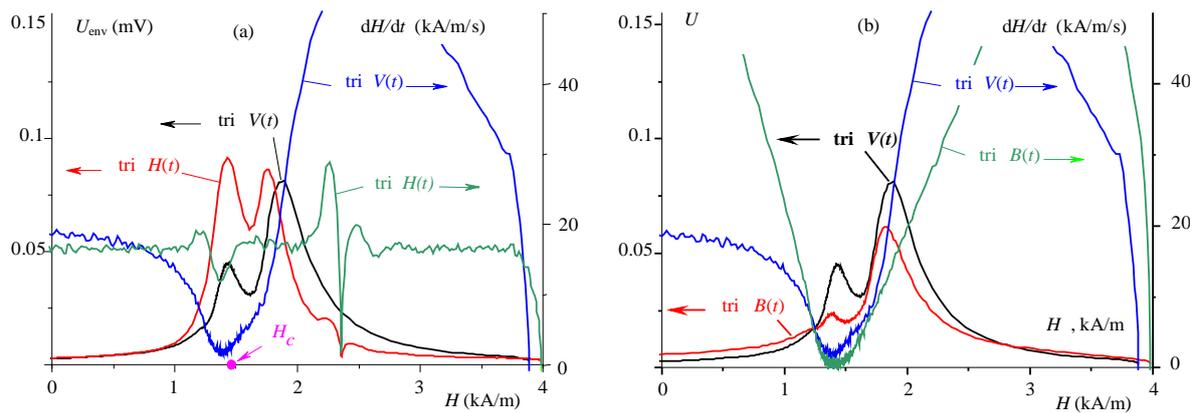
**Fig. 4.** The BN envelopes  $U_{env}$  (left scale, thick lines) and the corresponding field rates  $dH/dt$  (right scales, thin lines) as functions of the magnetic field  $H$ . The measurements were performed for the 100Cr6 bearing steel milled with  $VB = 0.2$  mm: (a) - with the triangular  $V(t)$  and  $H(t)$  waveforms; (b) - with the triangular  $V(t)$  and  $B(t)$  waveforms.
