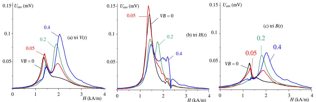
**Fig. 3.** The BN envelopes  $U_{env}$  for the milled 100Cr6 samples measured with the triangular waveforms of the magnetizing voltage  $V(t)$  - (a), the extrapolated field  $H(t)$  - (b) and the magnetic induction  $B(t)$  - (c). The flank wear  $VB = 0$  corresponds to the unmilled sample.
