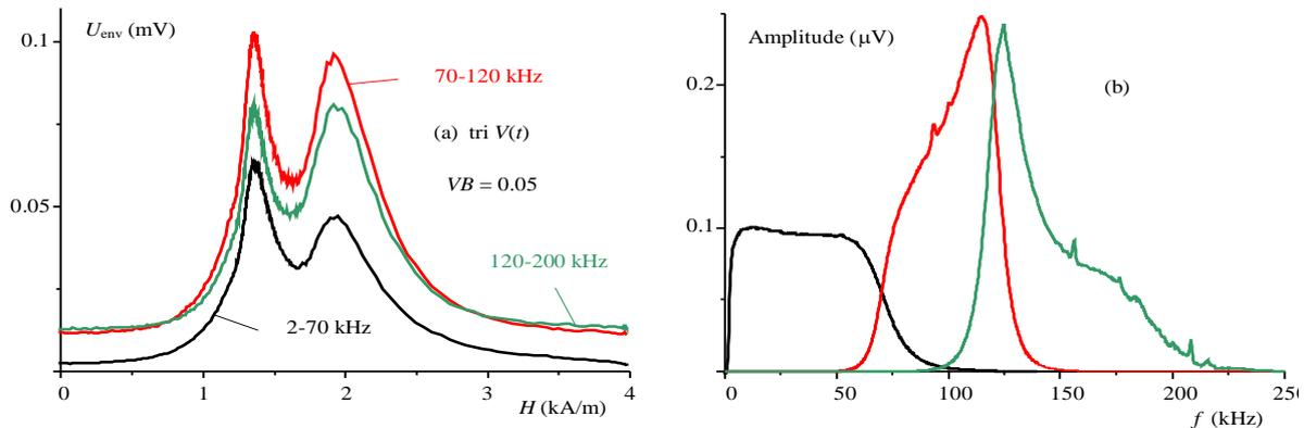
**Fig. 5.** (a) - The BN envelopes  $U_{env}$  for the 100Cr6 steel milled with  $VB = 0.05$  mm. The measurements were performed with the triangular  $V(t)$ ; the BN signal was filtered in the different bandwidths, (b) - The corresponding filtered spectra of the BN signal.
