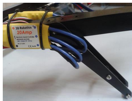
Fig. 2. Controller output wires on the arm of UAV
