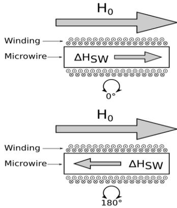
**Fig. 2.** Illustration of the fields before and after the turning of the sensor
