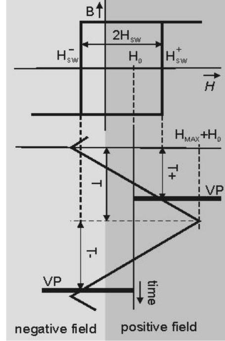
**Fig. 1.** Induction measurement method including offset of switching field
