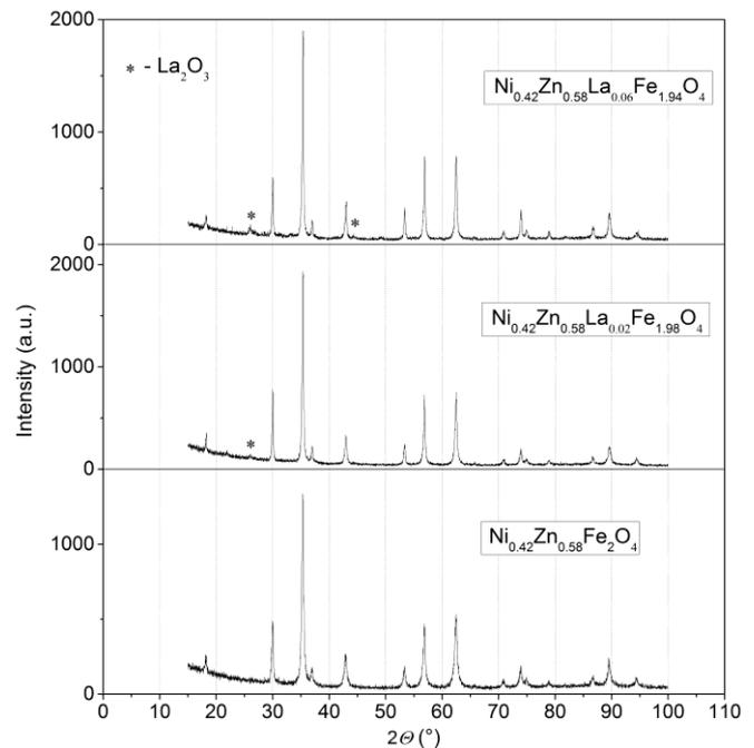
Fig. 2. XRD patterns of  $\text{Ni}_{0.42}\text{Zn}_{0.58}\text{La}_x\text{Fe}_{2-x}\text{O}_4$
