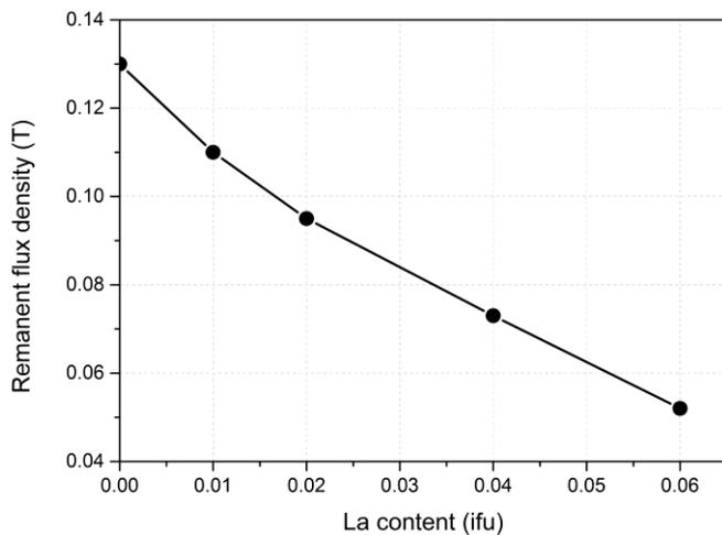
Fig. 5. Remanent flux density as a function of La content
