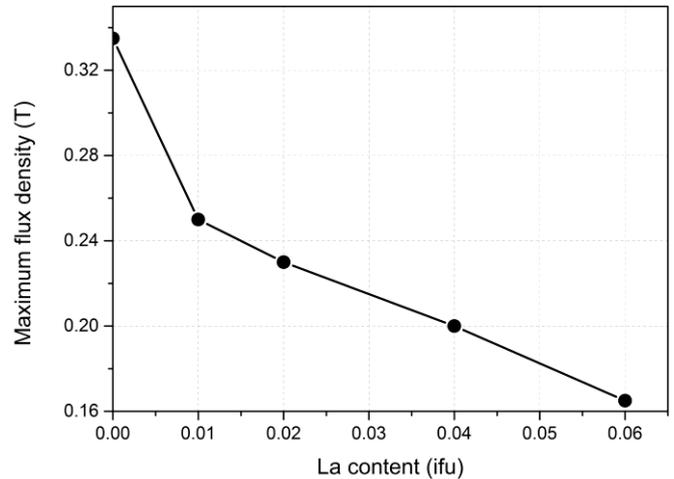
Fig. 6. Maximum flux density as a function of La content
