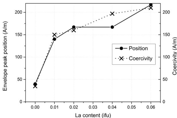
Fig. 9. La content dependence of MBN envelope peak position. Coercivity curve was added for comparison.
