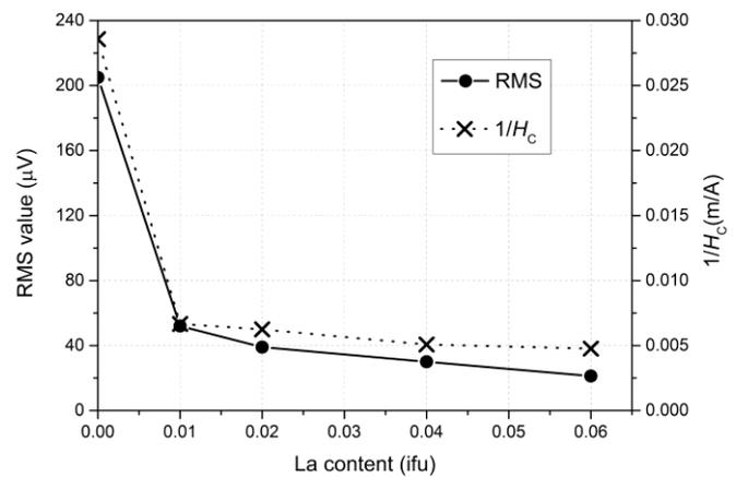
Fig. 7. La content dependence of MBN root mean square.  $1/H_c$  curve was added for comparison.
