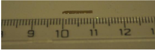
Fig. 1. Heusler alloy in the form of a ribbon
