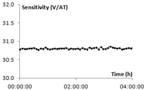
Fig. 7. Time drift of current-related sensitivity of developed graphene Hall-effect sensor
