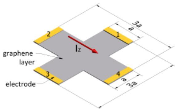
**Fig. 1.** Developed cross-shaped graphene Hall-effect structure,  $I_z$  – supply current flow direction, 1-4 – electrodes,  $a = 500 \mu\text{m}$
