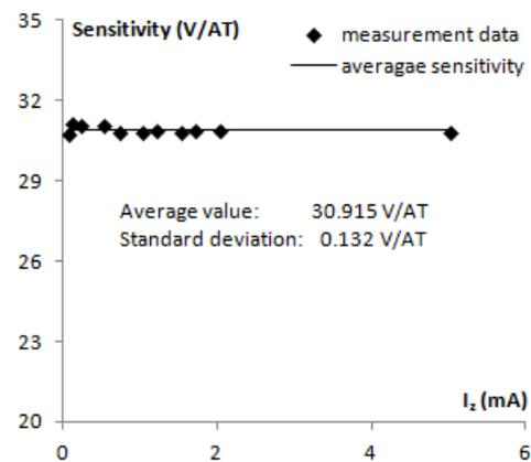
Fig. 5. Supply current  $I_z$  dependence of current-related sensitivity of developed graphene Hall-effect sensor
