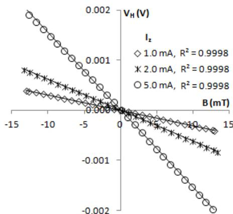
Fig. 4.  $V_H(B)$  characteristics of developed graphene Hall-effect sensor for several values of supply current  $I_z$
