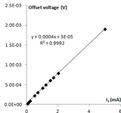
Fig. 6. Supply current  $I_z$  dependence of offset voltage of developed graphene Hall-effect sensor
