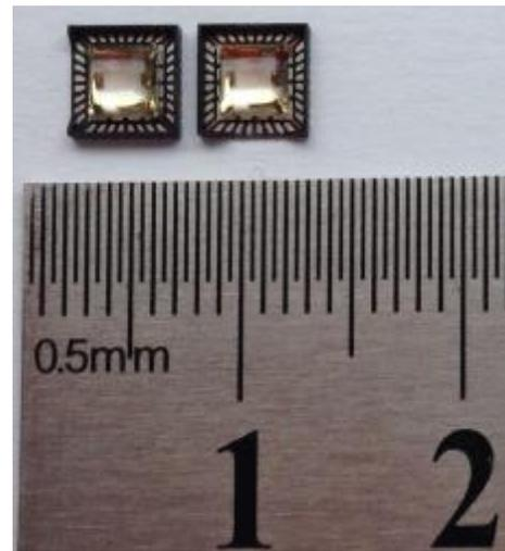
**Fig. 2.** Developed graphene Hall-effect sensors of magnetic field
