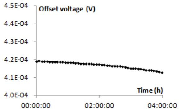
Fig. 8. Time drift of offset voltage of developed graphene Hall-effect sensor
