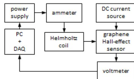
**Fig. 3.** Schematic block diagram of the measurement system
